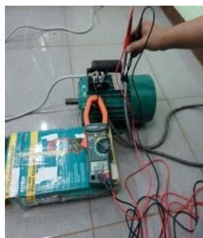
Figure 4 a. No-load induction motor test b. Locked-rotor induction motor test
